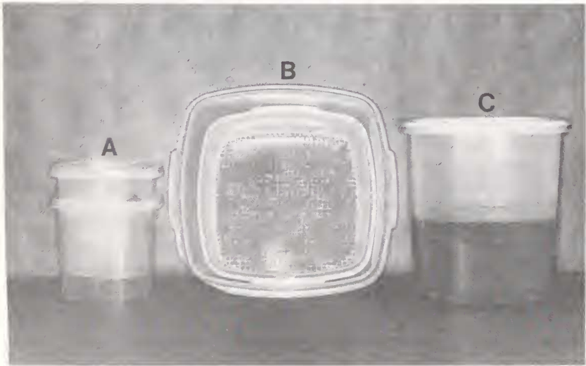
Figure 1. Apparatus used in separation procedure. From left to right are the fine mesh strainer (A), separation chamber (B), and transport/pouring container (C).
